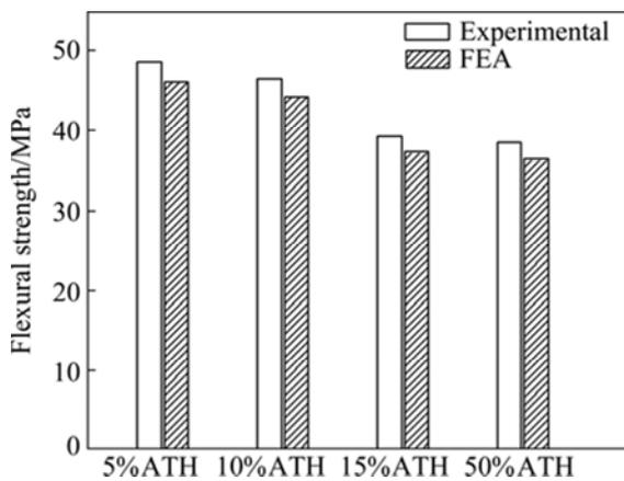
**Fig. 13** Comparison of FE and experimental values of flexural stress
