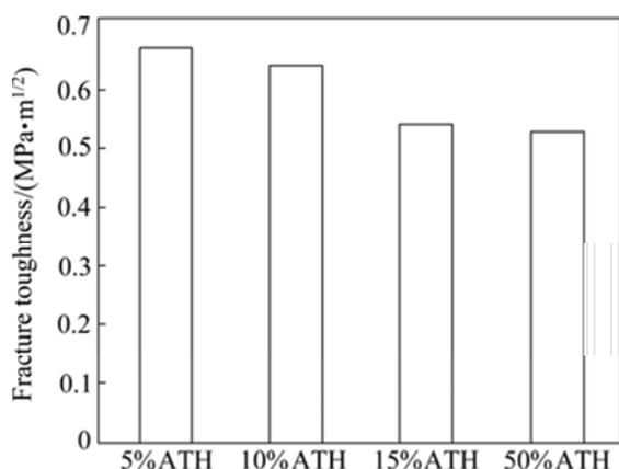
**Fig. 15** Variation of fracture toughness with different contents of ATH in PP/ATH composite
