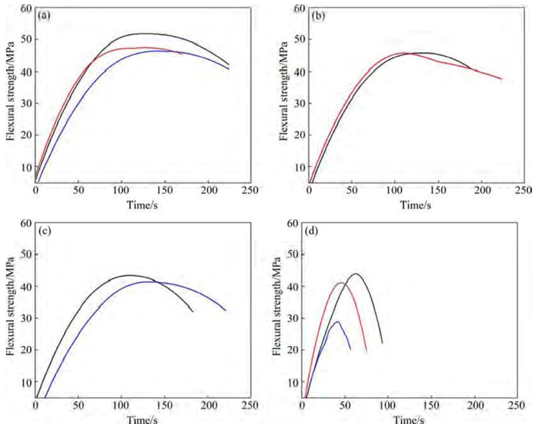
**Fig. 7** Flexural strength vs time plot for various blends of PP/ATH composite: (a) 5% ATH; (b) 10% ATH; (c) 15% ATH; (d) 50% ATH
