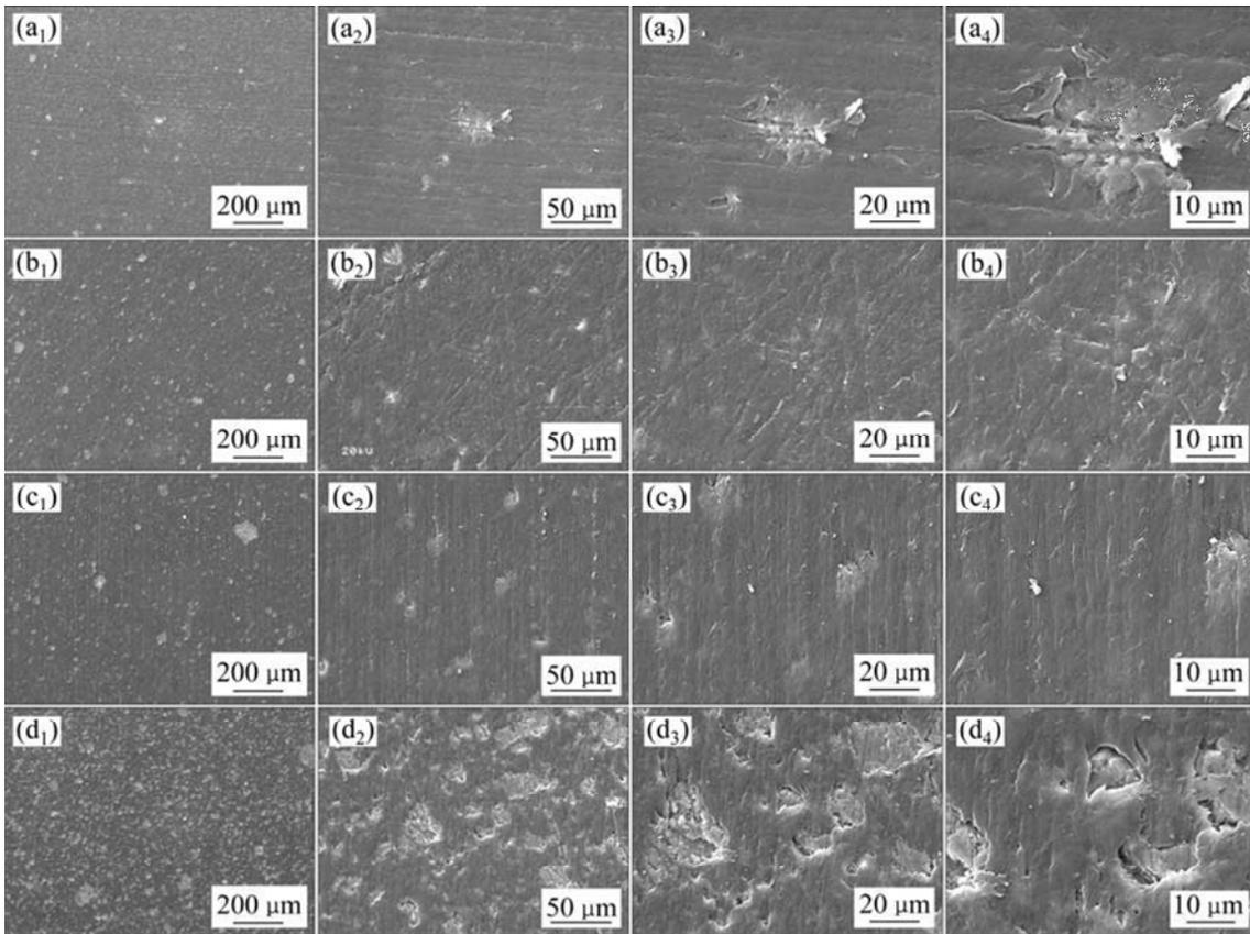
**Fig. 9** SEM images of PP/ATH composite specimens before loading: (a<sub>1</sub>)–(a<sub>4</sub>) PP+5%ATH; (b<sub>1</sub>)–(b<sub>4</sub>) PP+10%ATH; (c<sub>1</sub>)–(c<sub>4</sub>) PP+15%ATH; (d<sub>1</sub>)–(d<sub>4</sub>) PP+50%ATH
