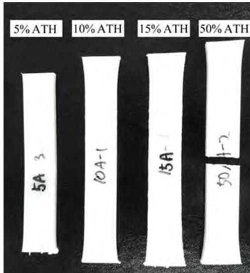
**Fig. 10** Camera image of specimens after bending test
