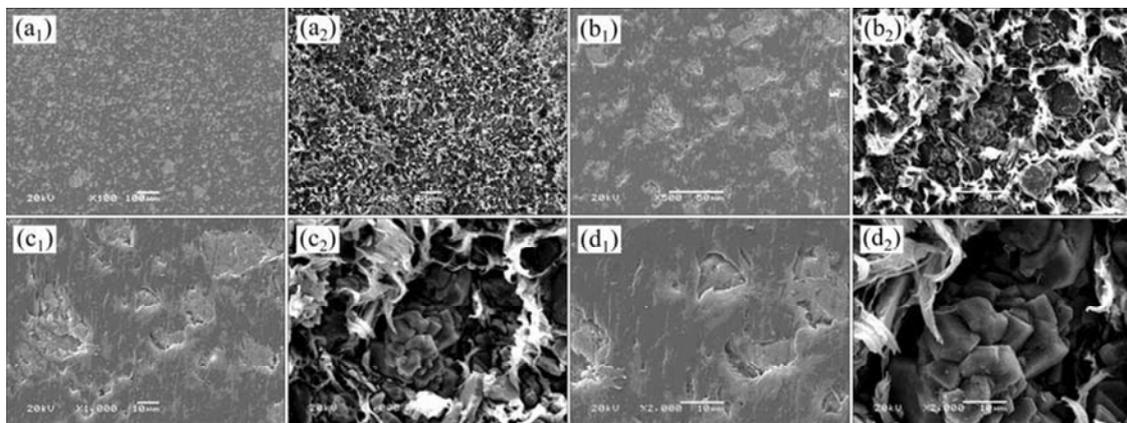
**Fig. 11** SEM images of fracture (50% ATH) specimen before loading (a<sub>1</sub>, b<sub>2</sub>, c<sub>3</sub>, d<sub>4</sub>) and after fracture (a<sub>2</sub>, b<sub>2</sub>, c<sub>2</sub>, d<sub>2</sub>): (a<sub>1</sub>, a<sub>2</sub>) 100x resolution; (b<sub>1</sub>, b<sub>2</sub>) 500x resolution; (c<sub>1</sub>, c<sub>2</sub>) 1000x resolution; (d<sub>1</sub>, d<sub>2</sub>) 2000x resolution
