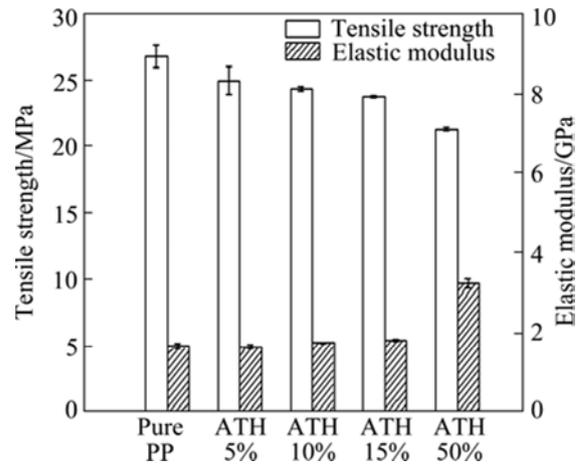
**Fig. 6** Variation in tensile strength and elastic modulus among different blends of PP/ATH
