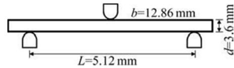
Fig. 3 Three-point bending test setup
