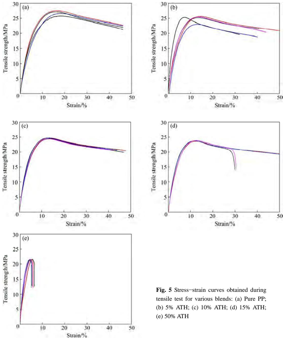
**Fig. 5** Stress–strain curves obtained during tensile test for various blends: (a) Pure PP; (b) 5% ATH; (c) 10% ATH; (d) 15% ATH; (e) 50% ATH
