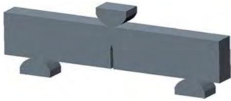
**Fig. 4** Geometric model for fracture analysis according to ASTM E1290
