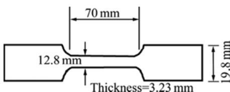
Fig. 2 Dog-bone specimen for tensile test
