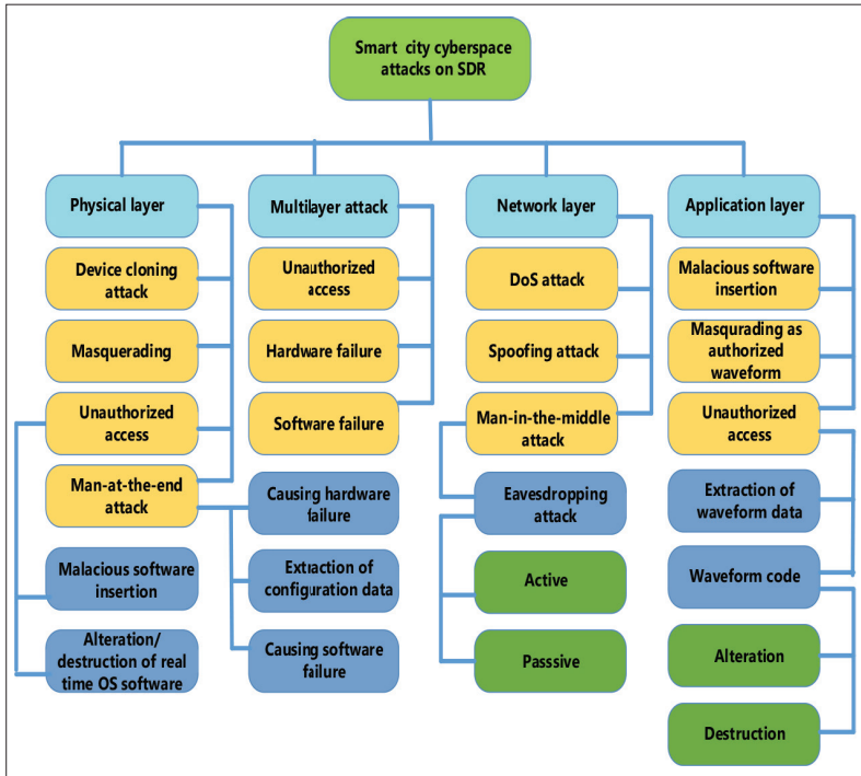
FIGURE 2. Taxonomy of SDR layered based security vulnerabilities, and attacks.
