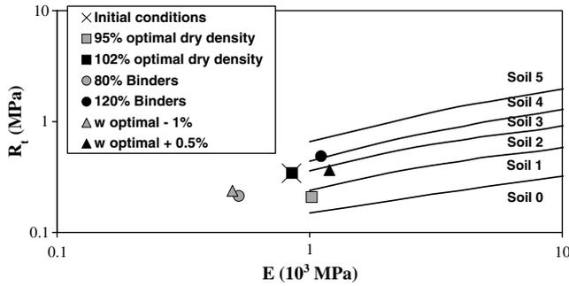
Fig. 8. Influence of the variability of dry density, binder proportion and water content on the mechanical behaviour of mix 1.
