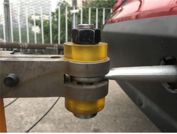
Fig. 11. Linkage between the test cart and the tractor.
