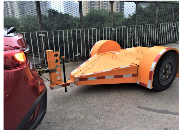
Fig. 9. Self-designed test vehicle resting on the bridge.
