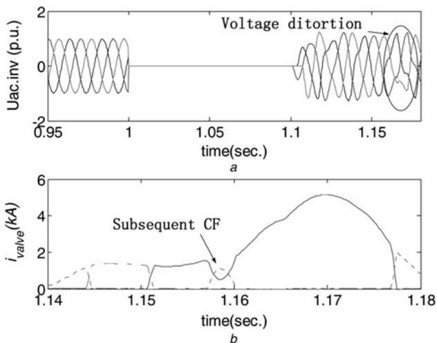
**Fig. 8** Instantaneous three-phase voltage and valve current under three-phase fault without VDDCFP ( $U_{ac,inv}$  is instantaneous three-phase voltage of AC system on the inverter side.  $i_{valve}$  is the valve current)
