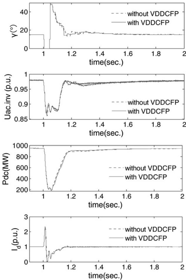
**Fig. 13** Inverter station II responses under single-phase fault in an AC system on the inverter I side ( $\gamma$  is the extinction angle on the inverter side.  $U_{ac,inv}$  is RMS voltage of AC system on the inverter side.  $P_{dc}$  is the HVDC power transmitted to the AC system.  $I_d$  is the direct current)
