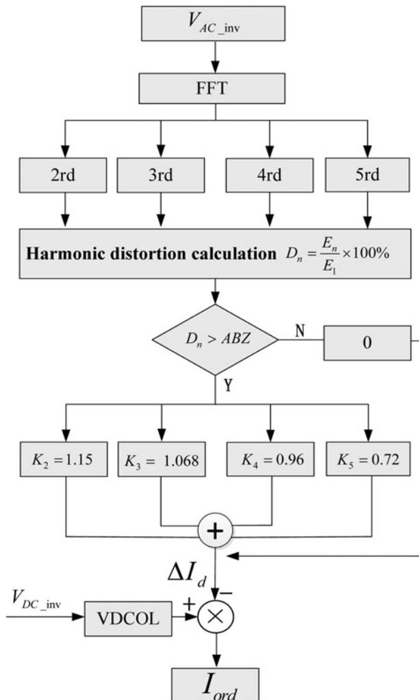
Fig. 6 Flow chart of VDDCFP controller in simulation model
