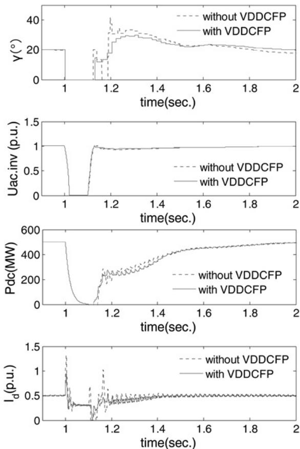
**Fig. 10** System response under three-phase fault in 50% power conditions ( $\gamma$  is the extinction angle on the inverter side.  $U_{ac,inv}$  is RMS voltage of AC system on the inverter side.  $P_{dc}$  is the HVDC power transmitted to the AC system.  $I_d$  is the direct current)
