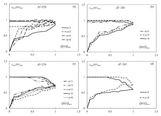
**Fig. 7.** Variation of maximum non-dimensional scour depth with non-dimensional discharge for different n values and non-dimensional time step discharge increase equal to: (a)  $\Delta T = 270$  and (b)  $\Delta T = 205$  (curved rock sill); (c)  $\Delta T = 270$  and (d)  $\Delta T = 205$  (straight rock sill).
