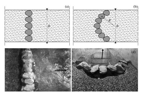
Fig. 2. (a) Diagram sketch and (c) picture of a straight rock sill; (b) Diagram sketch and (d) picture of a curved rock sill. The black arrow indicates the flow direction.
