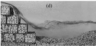
**Fig. 1.** Diagram sketch of a stepped gabion weir: (a) Nappe Flow, (b) Transition Flow, and (c) Skimming Flow regime; (d) picture of a stepped gabion weir.
