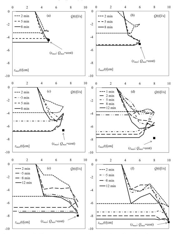
**Fig. 4.** Variation of scour depth evolution for different time step discharge increase along with the indication of the coordinates of maximum scour depth occurring for a steady test with discharge equal to  $Q_{max}$ . Peak discharge equal to: (a)  $Q_{max} = 5 \text{ l/s}$ ; (b)  $Q_{max} = 6 \text{ l/s}$ ; (c)  $Q_{max} = 7 \text{ l/s}$ ; (d)  $Q_{max} = 8 \text{ l/s}$ ; (e)  $Q_{max} = 9 \text{ l/s}$ ; (f)  $Q_{max} = 10 \text{ l/s}$ .
