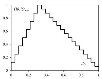
Fig. 3. Non-dimensional hydrograph adopted for tests with stepped gabion weirs.
