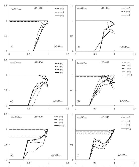
**Fig. 6.** Variation of maximum non-dimensional scour depth with non-dimensional discharge for different n values and non-dimensional time step discharge increase equal to: (a)  $\Delta T = 546$ ; (b)  $\Delta T = 484$ ; (c)  $\Delta T = 436$ ; (d)  $\Delta T = 400$ ; (e)  $\Delta T = 370$ ; (f)  $\Delta T = 345$ .
