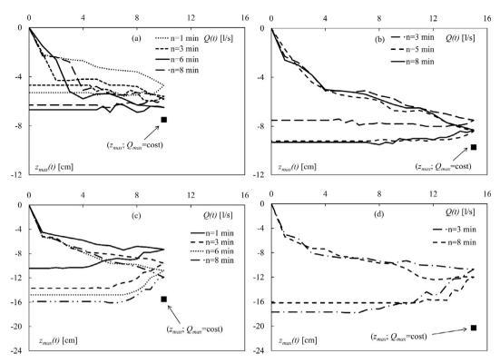
**Fig. 5.** Variation of scour depth evolution for different time step discharge increase along with the indication of the coordinates of maximum scour depth occurring for a steady test with discharge equal to  $Q_{max}$ . Peak discharge equal to: (a)  $Q_{max} = 10 \text{ l/s}$  and (b)  $Q_{max} = 15 \text{ l/s}$  (curved rock sill); (c)  $Q_{max} = 10 \text{ l/s}$  and  $Q_{max} = 15 \text{ l/s}$  (straight rock sill).
