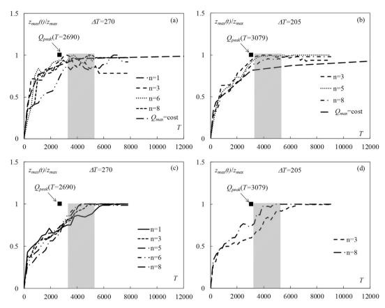
**Fig. 9.** Variation of maximum non-dimensional scour depth with non-dimensional time T for different n values and non-dimensional time step discharge increase along with the indication of the non-dimensional time T in which  $Q_{peak}$  is reached: (a)  $\Delta T = 270$  and (b)  $\Delta T = 205$  (curved rock sill); (c)  $\Delta T = 270$  and (d)  $\Delta T = 205$  (straight rock sill).
