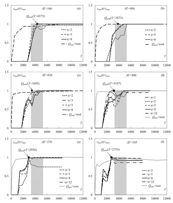
**Fig. 8.** Variation of maximum non-dimensional scour depth with non-dimensional time T for different n values and non-dimensional time step discharge increase along with the indication of the non-dimensional time T in which  $Q_{peak}$  is reached: (a)  $\Delta T = 546$ ; (b)  $\Delta T = 484$ ; (c)  $\Delta T = 436$ ; (d)  $\Delta T = 400$ ; (e)  $\Delta T = 370$ ; (f)  $\Delta T = 345$ .
