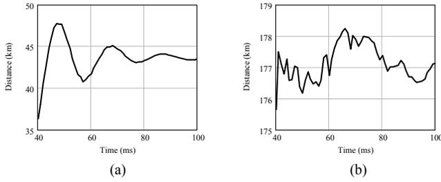
Fig. 6. Estimated fault distances for the assumption of the fault in front of (a) and behind (b) the compensation stage
