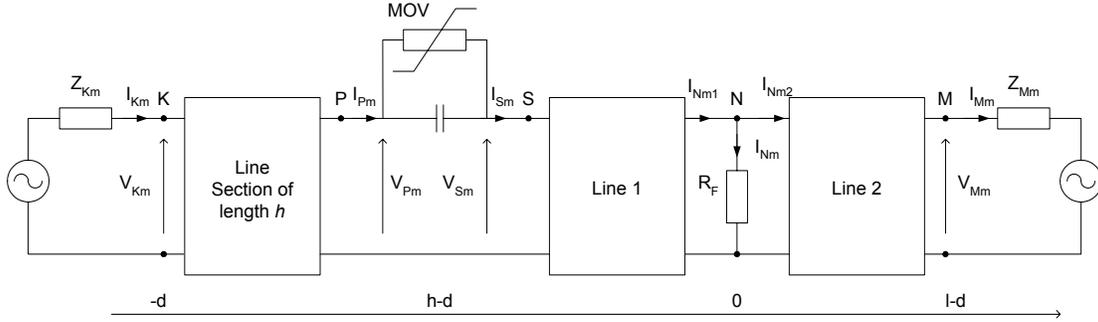
Fig. 3. Equivalent circuit of the series compensated line and source networks expressed in modal quantities.
