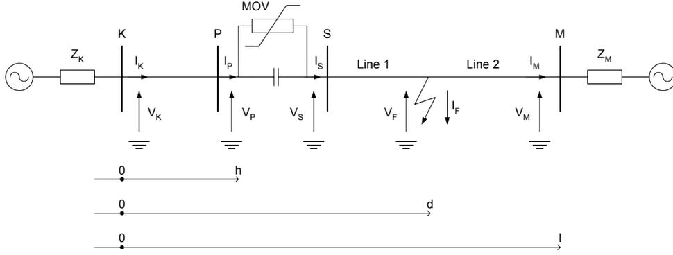
Fig. 2. Single-line diagram of a series compensated line with a fault at distance  $d$ .
