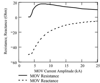
Fig. 4. Typical current-dependent characteristics of the impedance of the block capacitance-MOV
