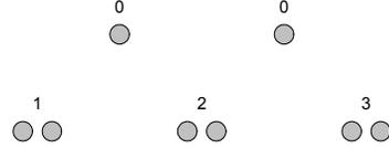
Fig. 5. 380-kV overhead line with two ground wires and 2-bundle phase wires
