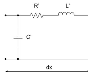
Fig. 1. An infinitesimal section of a single-phase homogeneous line.
