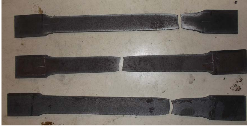
Figure 9. Three failed specimens under tensile loading
