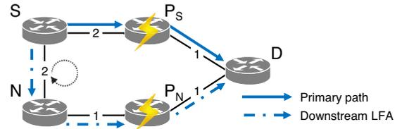
Fig. 3. Neighbor  $N$  is a downstream LFA of  $S$  but not vice-versa. The use of only downstream LFAs avoids loops in the presence of multiple failures.
