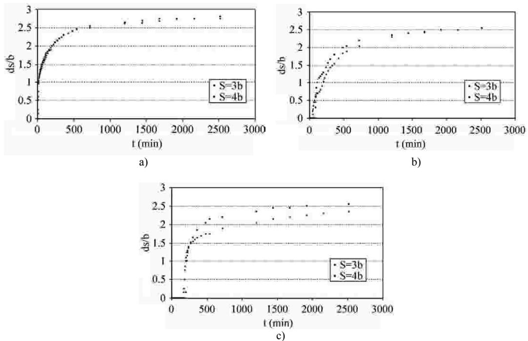
**Fig. 10** Time development of scour depth at group of three piers with collar
