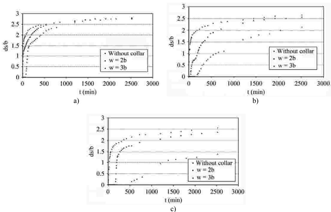
Fig. 9 Time development of scouring depth at group of three piers with and without collar
