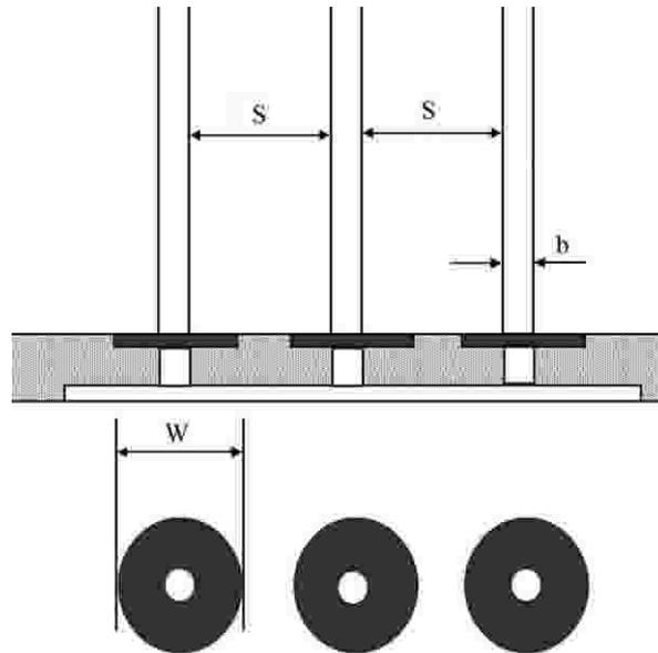
Fig. 3 Three piers in line with collar
