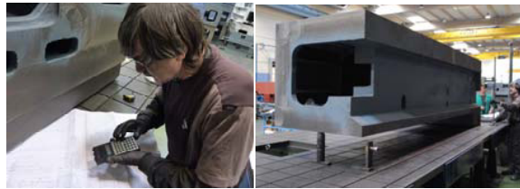
Fig. 1. Example of manual raw part fitting process: part setting calculation (left) and reference marking (right).
