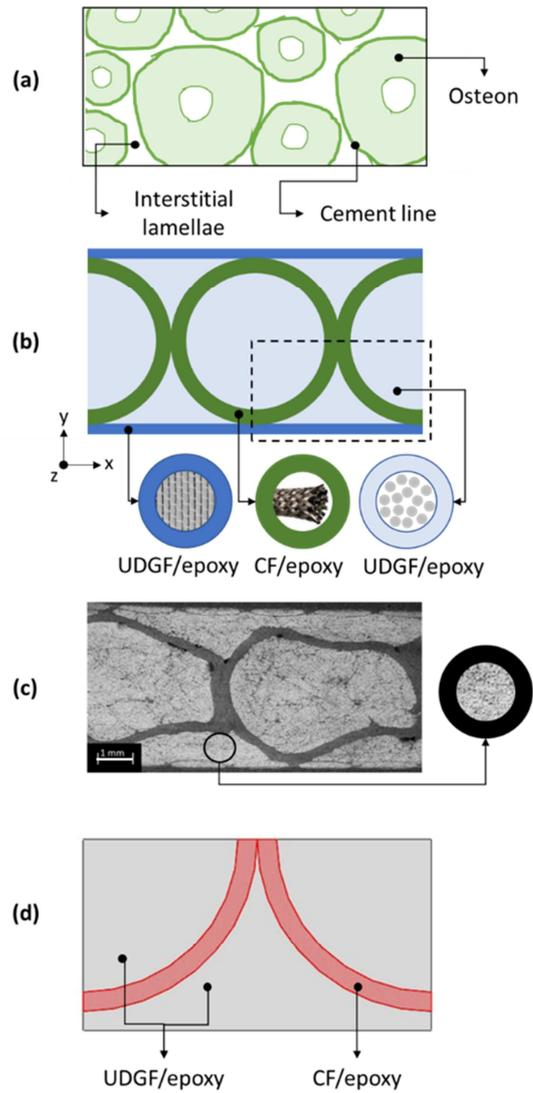
**Fig. 1.** (a) Schematic representation of the microstructure of cortical bone. (b) Schematic of the bioinspired design; the dashed area represents the repetitive unit. (c) SEM image showing the cross section of the previously developed bioinspired composite; scale bar 1mm. (d) Schematic of the modeled repetitive unit, highlighting the different subregions.
