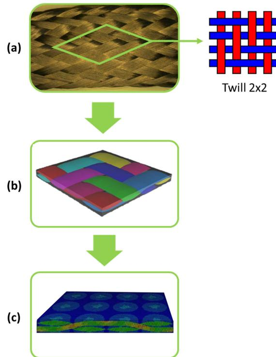
**Fig. 2.** Flow chart showing the steps followed to obtain the material properties of the CF-epoxy region. (a) Observation of the CF-sleeve by optical microscope and measurement of the yarn dimensions; highlighted the region of interest and, as magnification, a schematic of the fabric configuration (Twill 2x2). (b) Building of the unit cell model (geometry and mesh) in Texgen. (c) Simulations carried out on the unit cell to obtain the mechanical properties of the CF/epoxy region.
