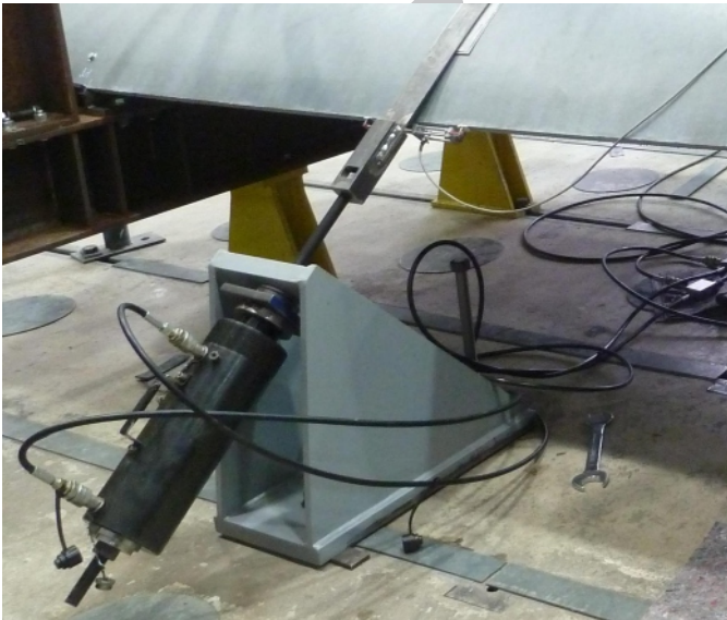
Figure 8: (a) test setup of the TRC vault shell with corresponding support conditions, loads and measuring points ; (b) test specimen in the laboratory and (c) detail of the hydraulic cylinder for the application of load S (bottom)
