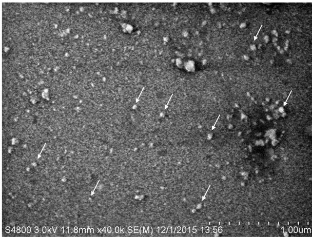
Fig. 10. Scanning electron microscopy (SEM) image of the three-component composite film made of PMMA and the nanoparticles of NaYF<sub>4</sub>: Yb<sup>3+</sup>, Er<sup>3+</sup> and AZO with magnification  $\times 40000$ . White arrows point to exemplary nanoparticles of various sizes embedded in the polymer matrix.
