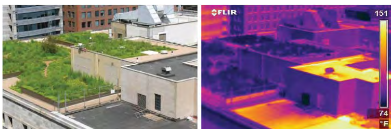
Figure 3: Thermal diagram of Chicago City hall. On a typical day, the green roof of the City Hall is about 40 degrees cooler than the surrounding areas.
