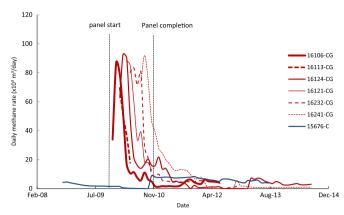
Fig. 7. Methane production profiles of GGVs during and after mining of the E-1 panel.
