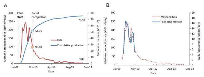
Fig. 8. Rate and cumulative methane production from all GGVs (a) and the correlation of mining advance rate to methane production rate (B).
