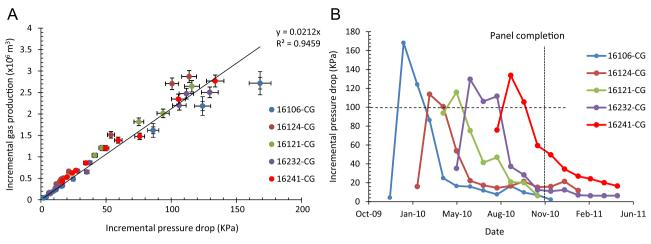
**Fig. 11.** Incremental gas production and formation pressure drop relation (A) and the history of change in pressure drop (B) during mining of the E-1 panel. The error bars in 10-A show 10% error margin of the value of the data points, whereas the 100 KPa level in B show the limit up to which the relation is linear for all GGVs.
