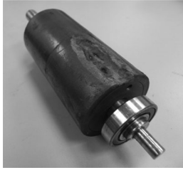
Fig. 24. Rotor with a single pole damaged to imitate partial demagnetization.
