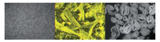
Fig. 3.2 A comparison of the structures of gel particles using CSLM (confocal scanning laser microscopy) (left), PCWM (centre) and crosslinked maize starch (right). Each image width is  $200\,\mu$ m.
