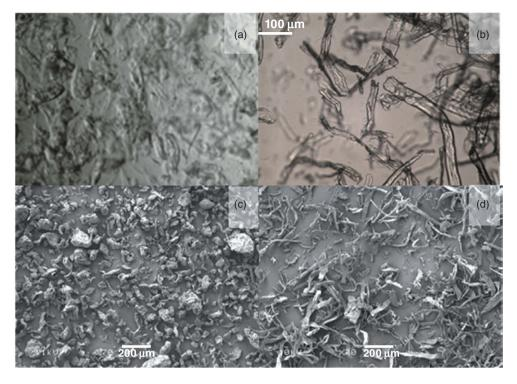
**Fig. 3.1** Hydrated (a and b) and dry (c and d) of citrus fibre (a and c) and powdered cellulose (b and d). The scale bar in b is common for both hydrated micrographs and that in the dry sample in 200 µm.
