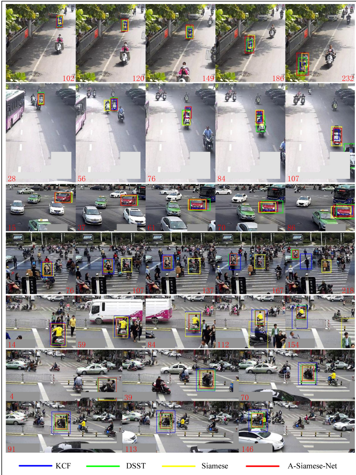
Figure 14. Tracking results on key frames in part of video sequences. When the target vehicle is far away from the camera, the KCF method cannot capture the features of the vehicle better. The Siamese method has a poor tracking result when the target vehicle is in a complex background area. Our SAS-Net has achieved good results compared with other methods.
