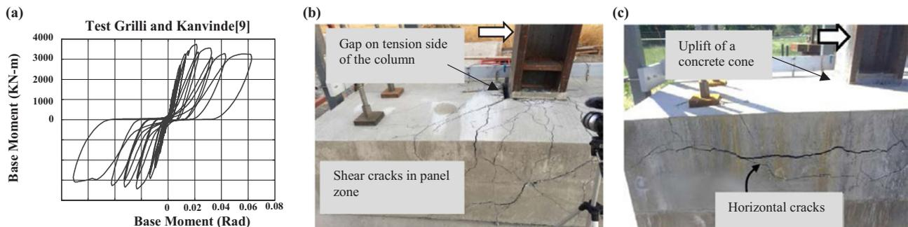
Fig. 2. Response of ECB: (a) Moment Rotation Response, (b) bearing cracking, (c) uplift failure.
