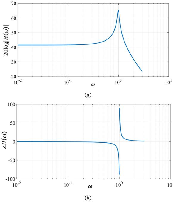
Fig. 3. Frequency response of the building under study to the base acceleration input in a logarithmic scale; (a) The magnitude part (in decibel) (b) The phase part (in degree).
