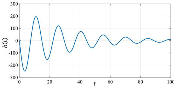
Fig. 4. Unit impulse response of the system due to the base acceleration input.
