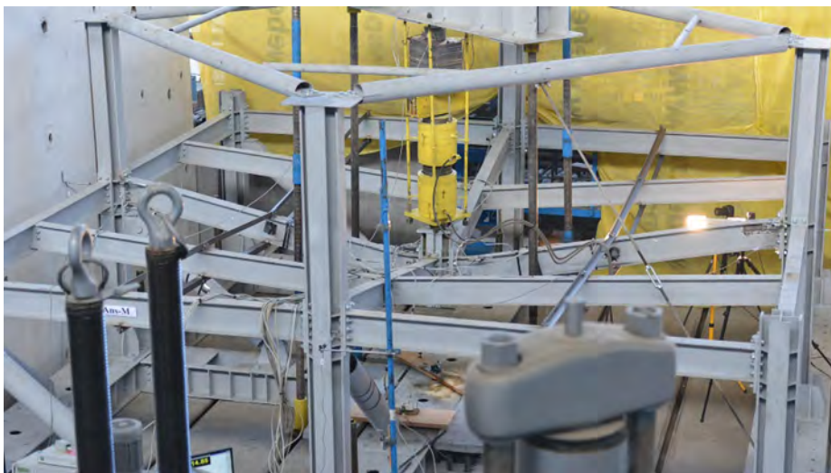
Fig. 13. Test on a 3D steel frame by Dinu et al. [204]. Photo by courtesy of Florea Dinu (Politehnica University Timisoara).
