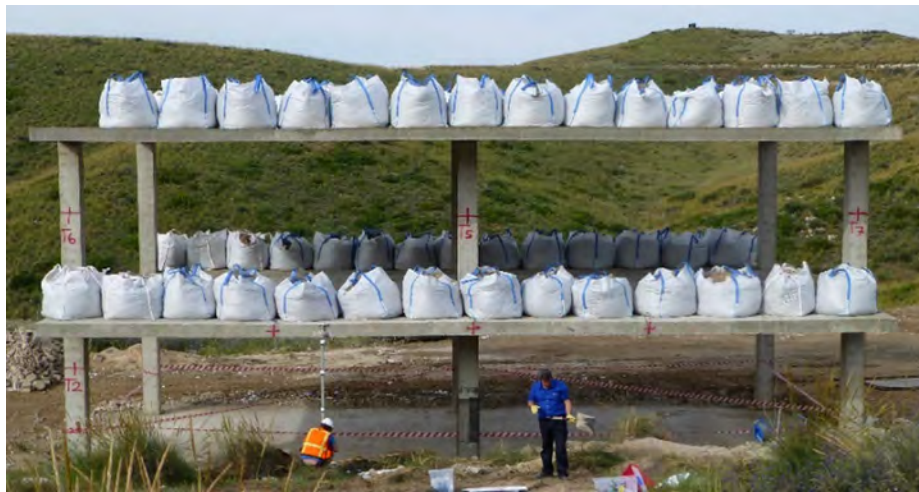
Fig. 14. Building structure tested by Bermejo et al. [207]. Photo by courtesy of Mario Bermejo (Technical University of Madrid).
