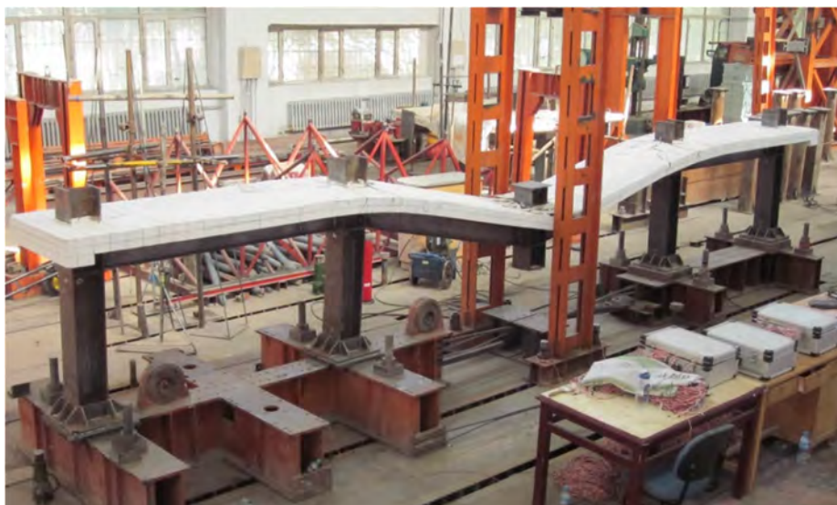
Fig. 11. View of a test by Guo et al. [195] on a composite frame. Photo by courtesy of Lanhui Guo (Harbin Institute of Technology).
