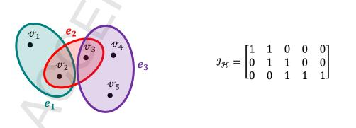
**Figure 4:** (a) Hypergraph; (b) Corresponding Incident matrix  $(\mathcal{I}_{\mathcal{H}})$
