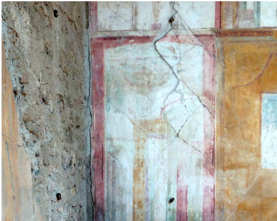
Fig. 3. Dataloggers (small black pieces) mounted at Ariadnas house at Pompeii (Italy).
