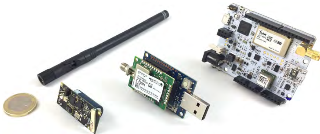
Fig. 6. Left: ITACA's custom node for 868 MHz ISM band. Central: LoRa compatible Multitech's .mDot evaluation kit. Right: Sigfox compatible Arrow's Smarteverything evaluation kit. Top: 4.5 dBi gain antenna.
