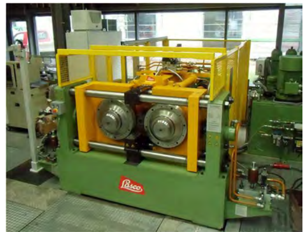
Fig. 31. Prototype machine for axial feed cross rolling [190].
