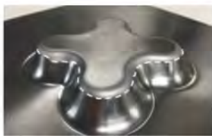
Fig. 6. Double sided incremental forming [145].
