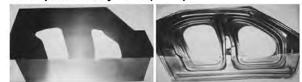
Fig. 37. Examples of the tailor welded blanks [132].
