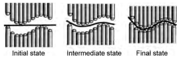
Fig. 61. Flexible forming with digitized die [112].
