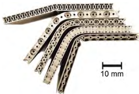
Fig. 39. Metallic sandwich sheets manufactured by selective laser melting with different core structures after bending to the same bending angle showing different spring-back.
