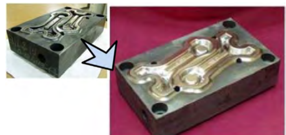
Fig. 41. Restoration of hot forging tools using laser assisted material deposition [3].
