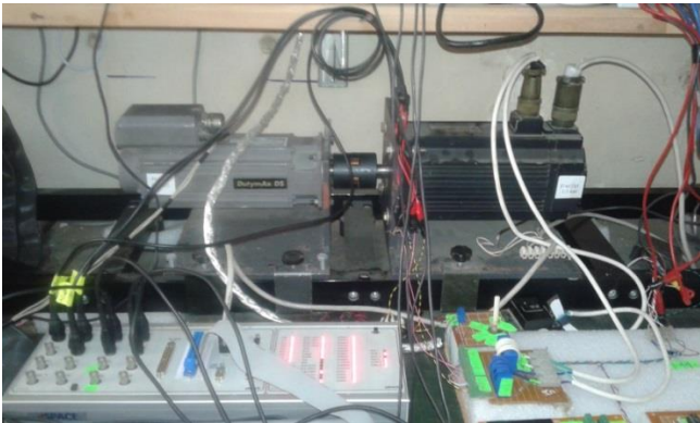
Fig. 10 Experimental setup for WTE using PMSM loaded with PMSG
