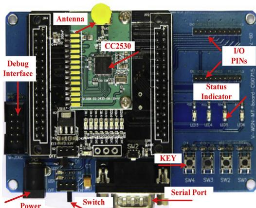
Fig. 3 – Appearance of motherboard for WSN nodes.
