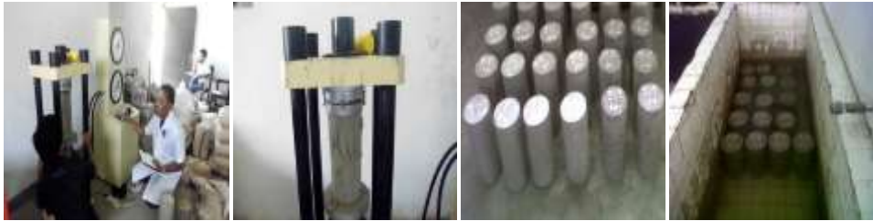
Figure 1. Compressive strength test process
