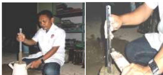
Figure 6. Slump test of fresh concrete from organic cement and concrete portland cement
