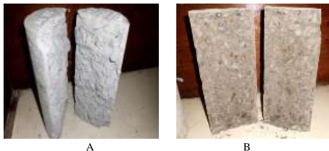
Figure 5. Cylinder concrete with organic cement from tensile splitting test (A), Cylinder concrete with portland cement from tensile splitting test (B)
