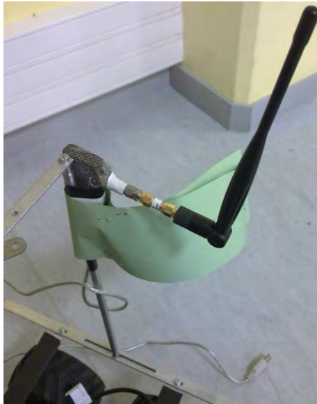
Figure 22: Fixed Radio Signal Attenuator on ARUM Mobile Node
