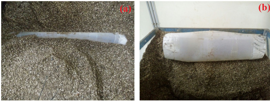
Fig. 10. T_{(t=1.0)} after test (a) tunnel embedded in soil, and (b) tunnel out of soil.
