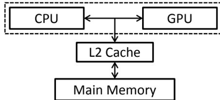
Figure 1: Overview of the coupled CPU-GPU architecture.
