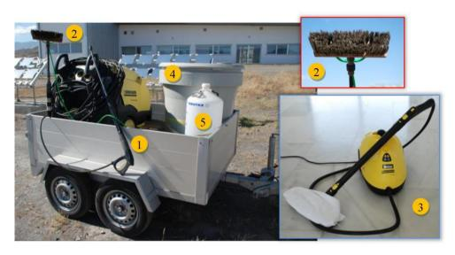
Fig. 4. Pressure washing device with hand spray nozzle accessory (1), water-fed natural horse-hair bristle brush accessory (2), steam cleaner (3), demineralized water tank (4), and additives tank (5).
