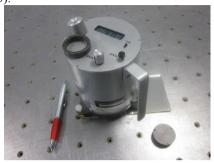
Fig. 3. Portable specular reflectometer 15R-USB by Devices and Services.
