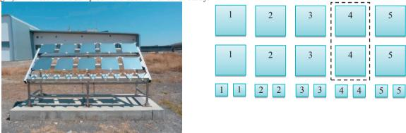
Fig. 2. Structure 2 (left) and distribution of solar reflectors per type in a test bench (right).
