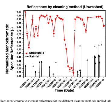
Fig. 6. Normalized monochromatic specular reflectance for the different cleaning methods applied, after cleaning (structure 4).
