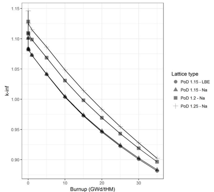
Fig. 3.  $k$ -inf as a function of burnup and Pitch over Diameter, with classification by coolant type.
