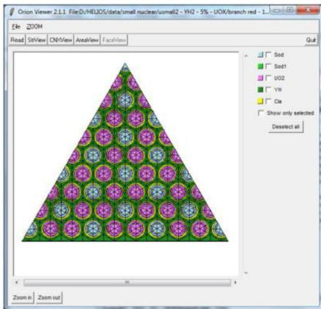
Fig. 2. Adapted fuel assembly with 5% enriched  $\text{UO}_2$  fuel.
