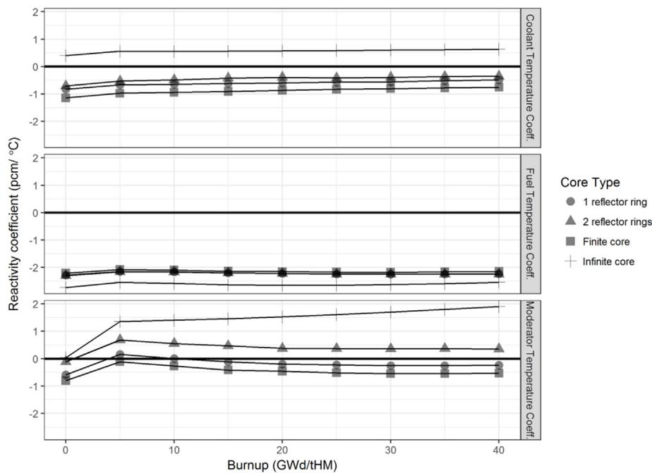
Fig. 10. Comparison of coolant, moderator and fuel temperature coefficients for the four core models of the micro-reactor.
