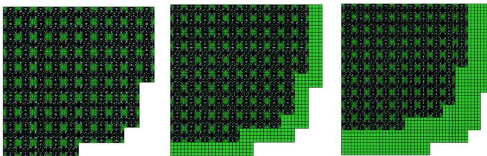
Fig. 8. From left to right: unreflected core (infinite and finite); reflected core with one reflector ring; and reflected core with two reflector rings.
