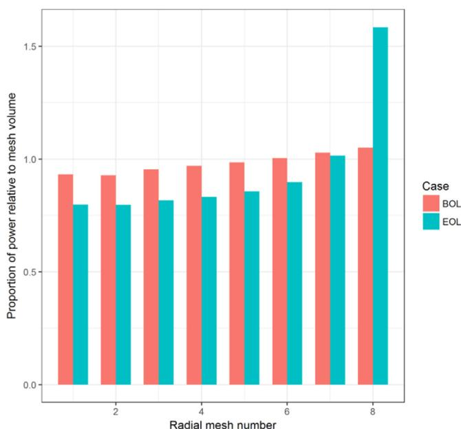
Fig. 7. Proportion of power relative to mesh volume for the unit cell shown in Fig. 5.
