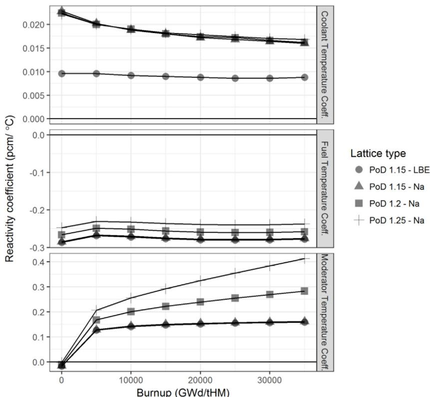
Fig. 4. Comparison of coolant, moderator and fuel temperature coefficients as a function of Pitch over Diameter and coolant type.
