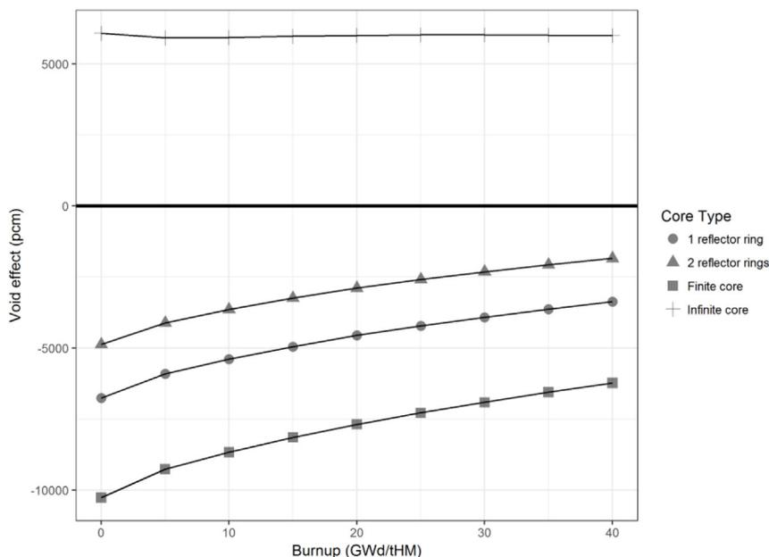
Fig. 9. Void effect by core type as a function of burnup.
