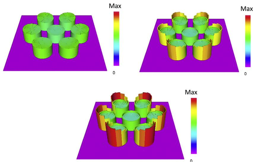
Fig. 6. Power distribution within the new unit cell configuration at 0, 20 and 40 GWd/tHM (left to right and top to bottom).
