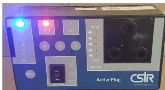
Figure 5 Constrained Application Protocol Sensing Device (ActivePlug)
