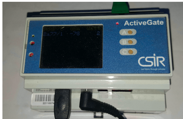
Figure 4 Constrained Application Protocol Gateway (ActiveGate)
