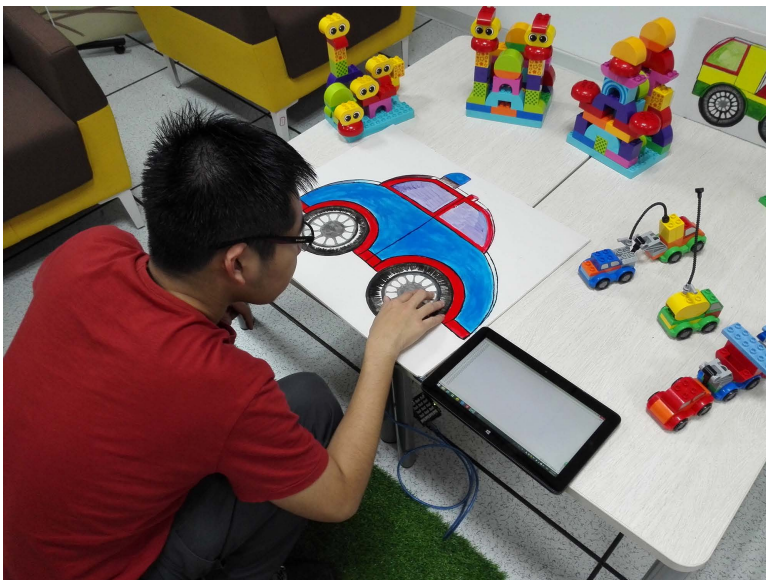
Figure 20.10 The play scenario where the tester is observed triggering the capacitive sensors.
