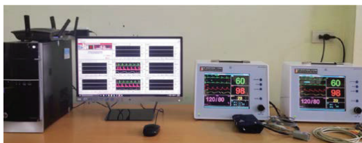
Figure 9. The single transmitter prototype to acquire and transmit data from the patient monitor devices
