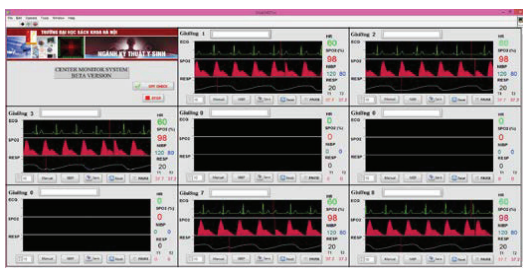
Figure 10. The central display software interface for 8 real-time data channels from 8 different patient monitor devices
