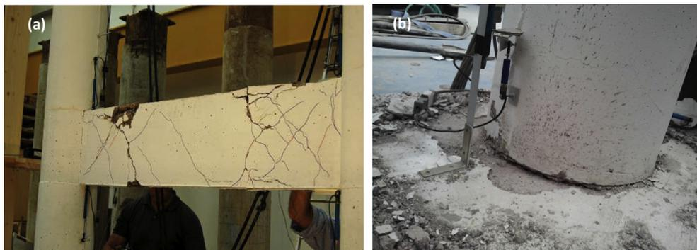
Fig. 6. Typical shear and flexural damage occurred respectively in the transverse beams and column of the experimental scaled model (after [55]).
