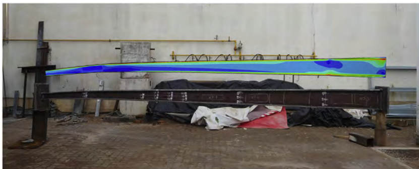
Fig. 39. Column 3: numerical and experimental deformed shape.
