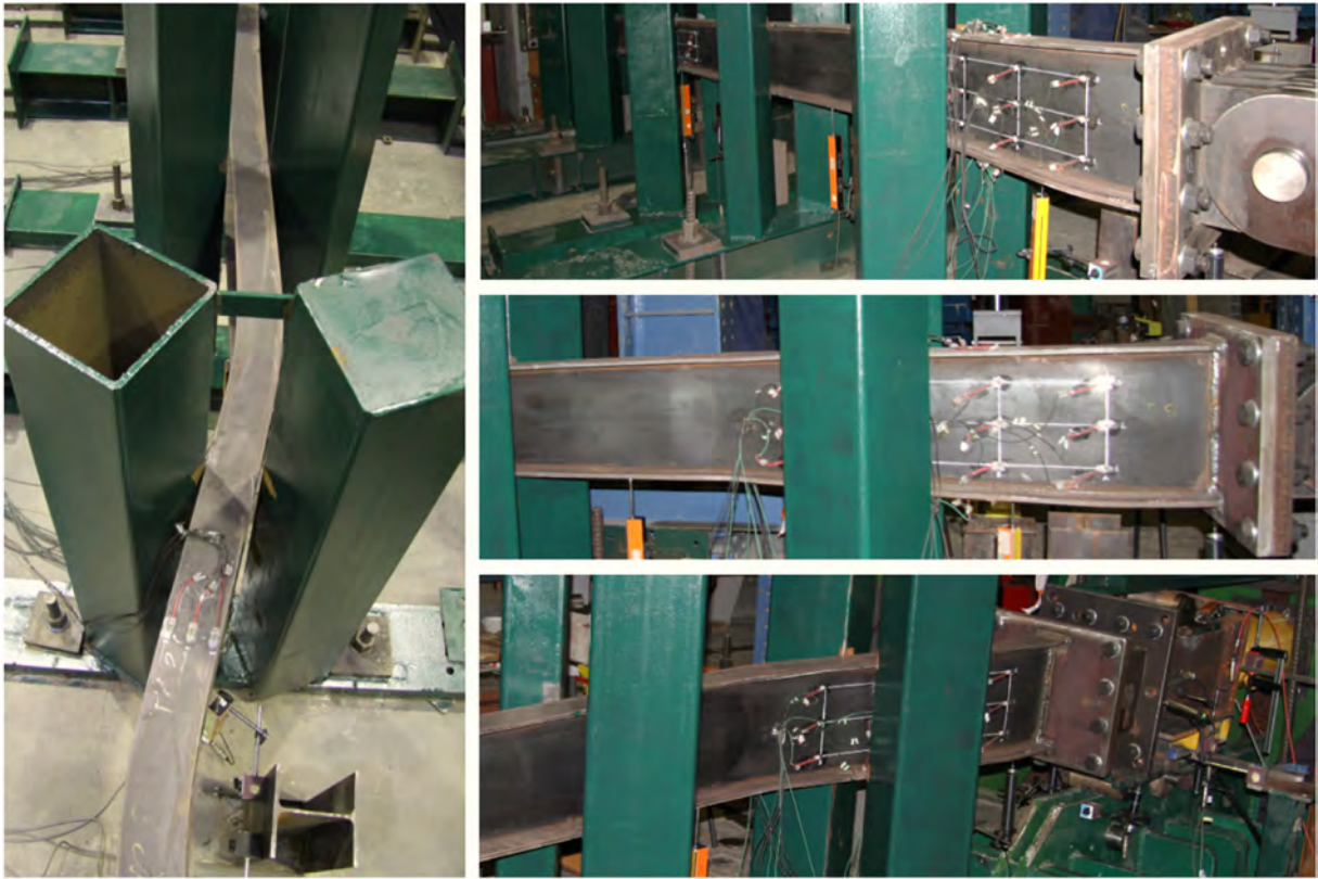
Fig. 19. Collapse of C2.
