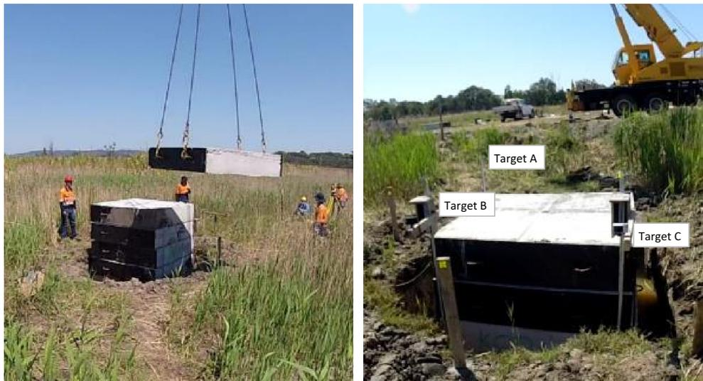
Fig. 13. Loading procedure of the unconsolidated undrained foundation tests (UU1 and UU2).
