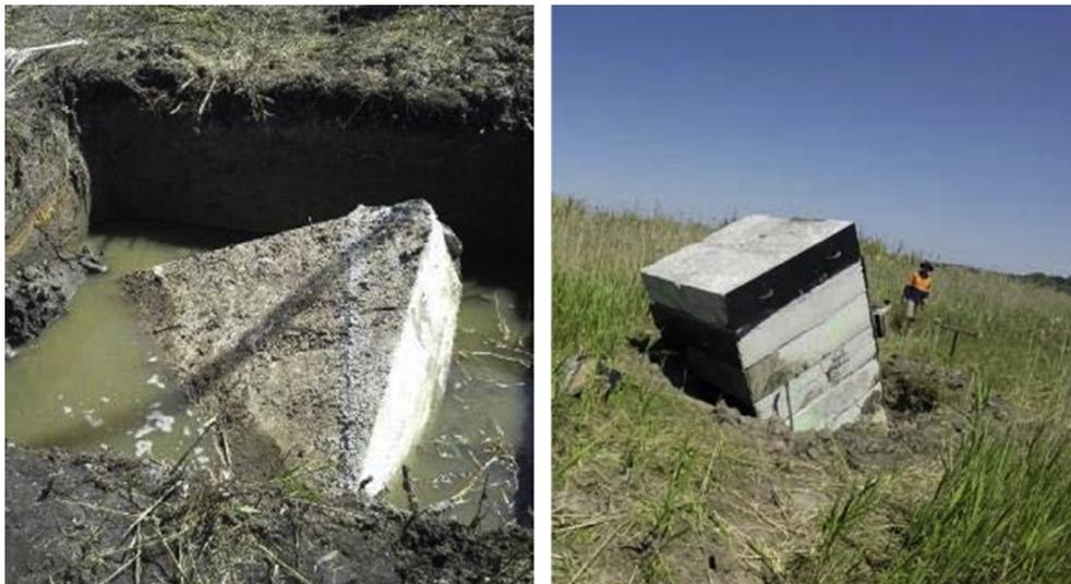
Fig. 17. Failure modes of the unconsolidated undrained foundation tests (left: UU1 and right: UU2).
