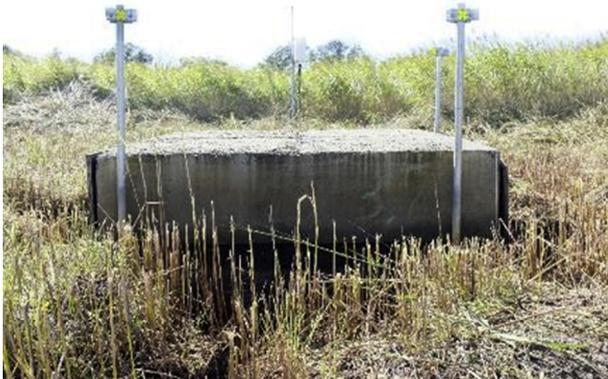
**Fig. 9.** Survey target set up for monitoring foundation displacements.
