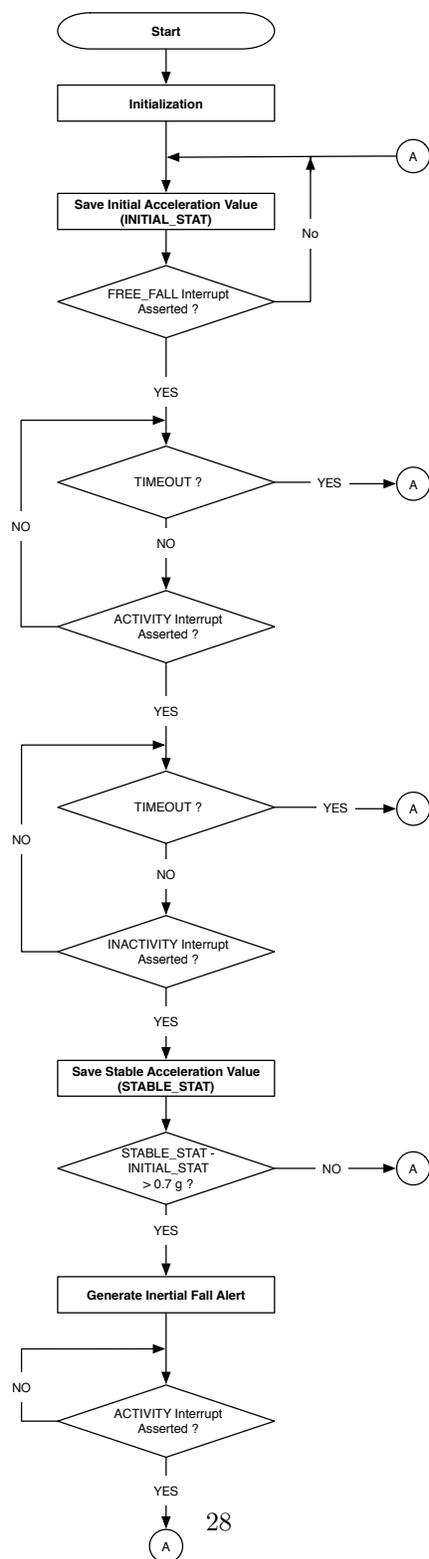
Figure 11: ADXL345-based Fall Detection Algorithm
