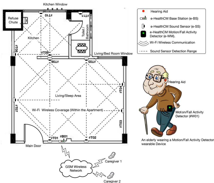
Figure 4: Healthcare-based e-HealthCM System Implemented in an apartment for the elderly
