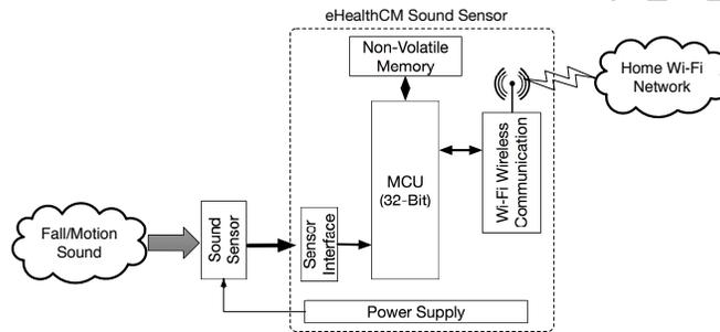
Figure 2: e-HealthCM Sound Sensor Hardware Block Diagram.
