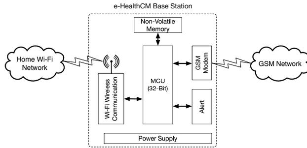
Figure 1: e-HealthCM Base Station Hardware Block Diagram.
