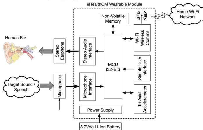
Figure 3: e-HealthCM Wearable Module Hardware Block Diagram.
