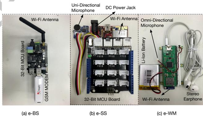
Figure 5: e-HealthCM Hardware Prototypes depicting (a) e-BS, (b) e-SS, and (c) e-WM.
