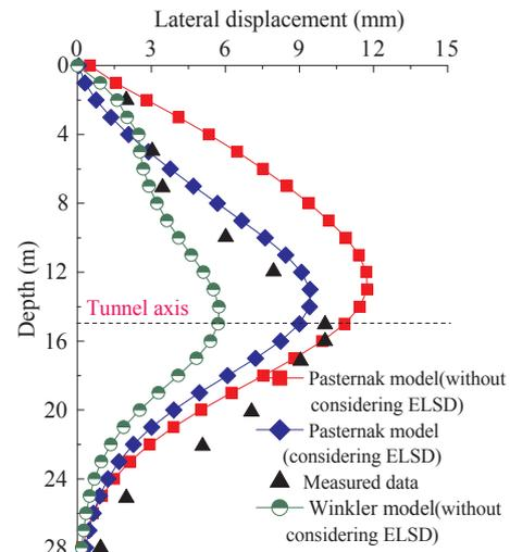
Fig. 8. Comparison of pile lateral displacement in case 2.
