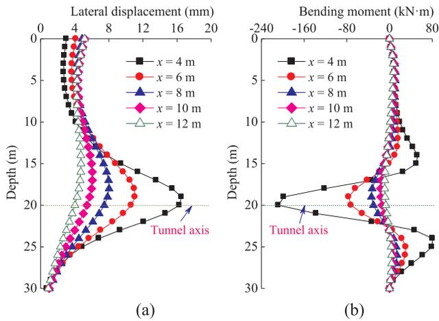
Fig. 12. Lateral displacement and bending moment of pile with different tunnel-pile distance: (a) lateral displacement; (b) bending moment.
