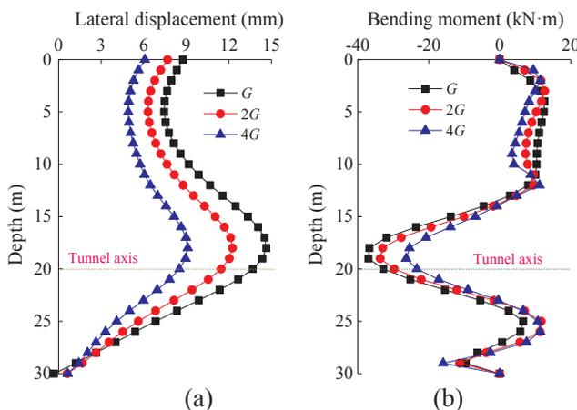
Fig. 17. Lateral displacement and bending moment of rear pile with different foundation shear modulus: (a) lateral displacement; (b) bending moment.
