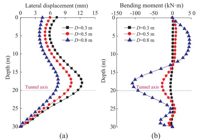
Fig. 19. Lateral displacement and bending moment of rear pile with different pile diameters: (a) lateral displacement; (b) bending moment.
