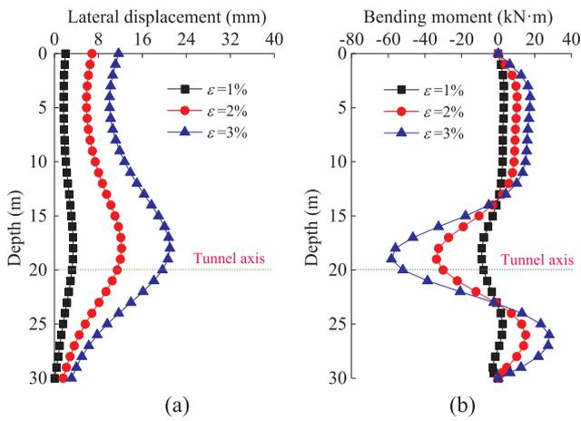
Fig. 21. Lateral displacement and bending moment of rear pile with different ground loss: (a) lateral displacement; (b) bending moment.
