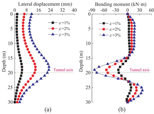
Fig. 20. Lateral displacement and bending moment of front pile with different ground loss: (a) lateral displacement; (b) bending moment.
