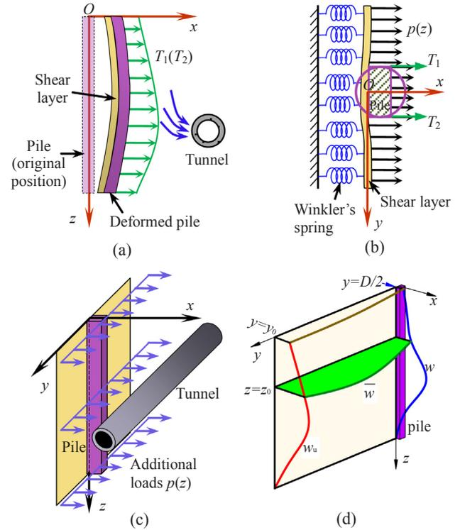
Fig. 5. Effects of lateral soils on piles: (a) deformed piles induced by lateral forces; (b) forces on piles delivered by shear layer; (c) additional loads applied on piles and lateral soils; (d) deformation of shear layer beside piles.
