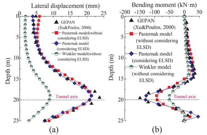
Fig. 7. Comparison of pile lateral displacement and bending moment in case 1: (a) lateral displacement and (b) bending moment.
