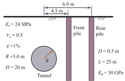
Fig. 13. Calculating diagram for the effect of  $2 \times 1$  pile group due to tunnelling (Loganathan et al., 2001).
