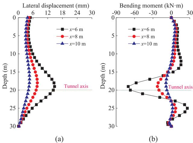
Fig. 22. Lateral displacement and bending moment of front pile with different pile-tunnel distance: (a) lateral displacement; (b) bending moment.
