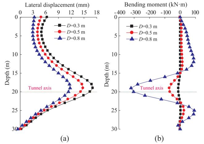
Fig. 18. Lateral displacement and bending moment of front pile with different pile diameters: (a) lateral displacement; (b) bending moment.
