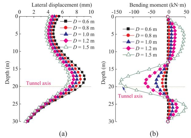
Fig. 10. Lateral displacement and bending moment of pile with different pile diameters: (a) lateral displacement; (b) bending moment.
