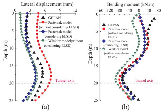
Fig. 15. Comparison of lateral displacement and bending moment of rear pile in case 4: (a) lateral displacement; (b) bending moment.
