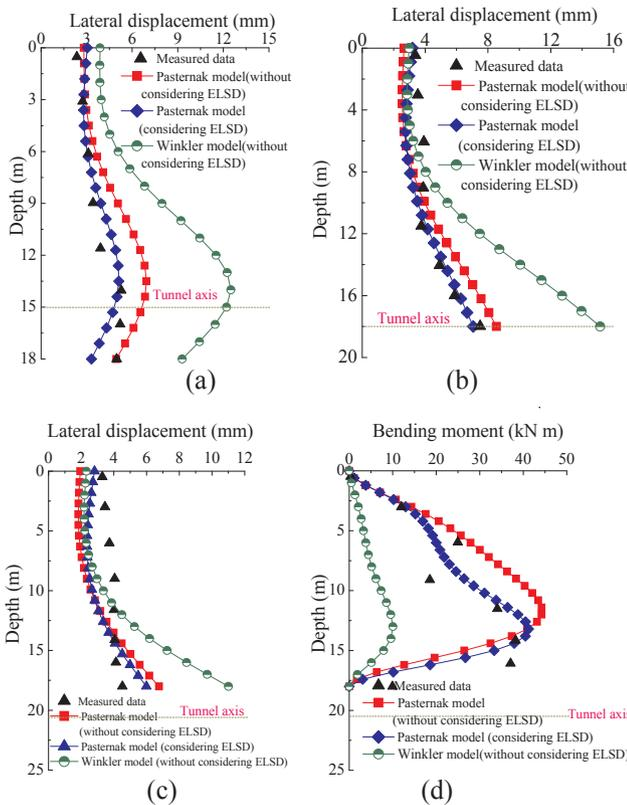
Fig. 9. Comparison of pile lateral displacement and bending moment in case 3: (a) lateral displacement in test 1; (b) lateral displacement in test 2; (c) lateral displacement in test 3; (d) bending moment in test 3.
