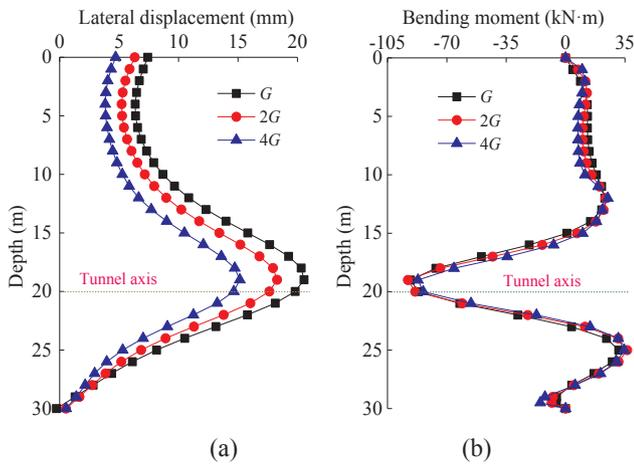
Fig. 16. Lateral displacement and bending moment of front pile with different foundation shear modulus: (a) lateral displacement; (b) bending moment.
