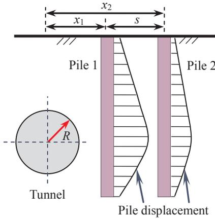
Fig. 4. Computing model for group-piles adjacent to tunnelling.
