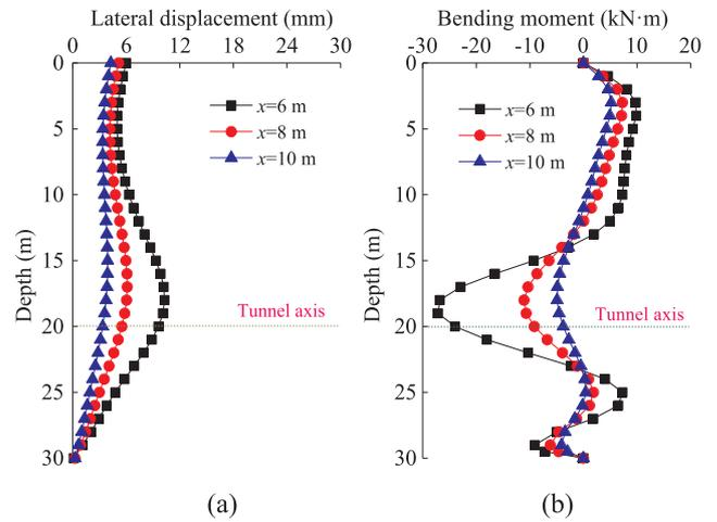
Fig. 23. Lateral displacement and bending moment of rear pile with different pile-tunnel distance: (a) lateral displacement; (b) bending moment.
