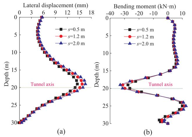
Fig. 24. Lateral displacement and bending moment of front pile with different pile spacing: (a) lateral displacement; (b) bending moment.
