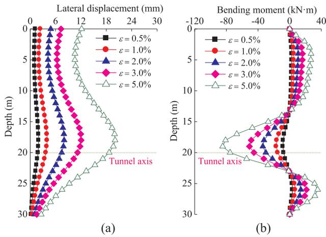
Fig. 11. Lateral displacement and bending moment of pile with different ground loss: (a) lateral displacement; (b) bending moment.
