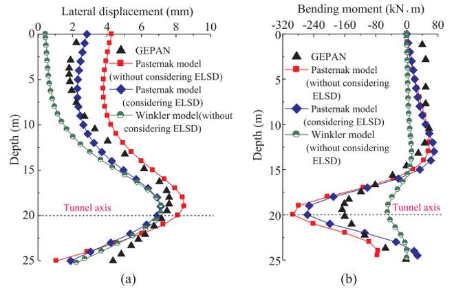
Fig. 14. Comparison of lateral displacement and bending moment of front pile in case 4: (a) lateral displacement; (b) bending moment.
