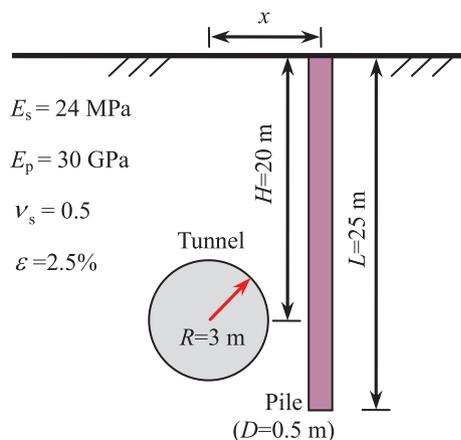
Fig. 6. Calculating diagram for effects of single-pile due to tunnelling (Xu and Poulos, 2001).
