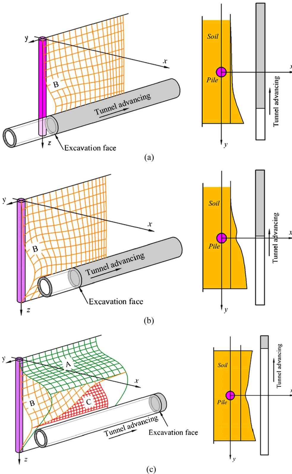
Fig. 2. Schematic view for effects of tunnelling on nearby piles: (a) short-range excavated; (b) medium-range excavated; (c) fully excavated.
