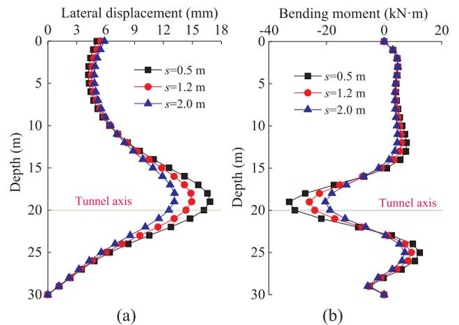
Fig. 25. Lateral displacement and bending moment of rear pile with different pile spacing: (a) lateral displacement; (b) bending moment.
