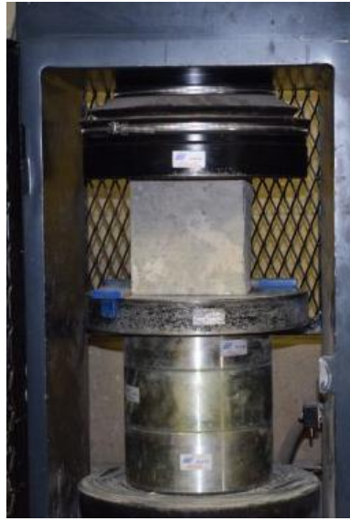
Figure 3. Compressive strength test of concrete cubic specimen.
