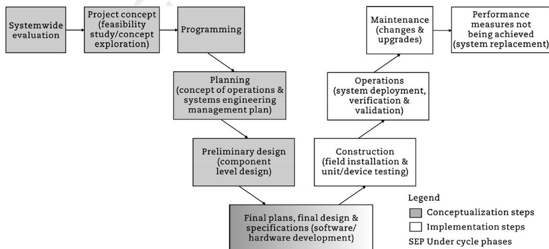
Fig. 2 – TSM&O project cycle diagram–high level diagram with system engineering process (SEP).
