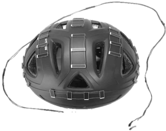
Fig. 3. PV Cells mounting on the cyclist helmet.
