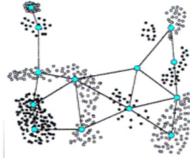
Fig. 3. Example of clustering data using growing neural gas
