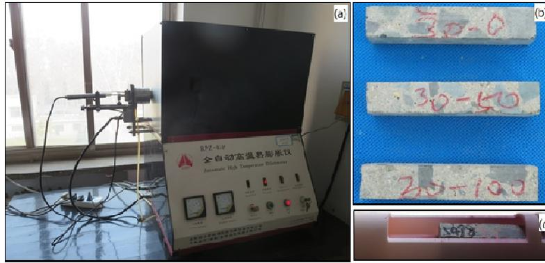
Fig. 3. Measurement of thermal expansion of coarse RCA concrete at elevated temperatures, (a) RPZ-03P Automatic High Temperature Dilatometer, (b) Concrete specimens, (c) Concrete specimen ready for thermal expansion tests.
