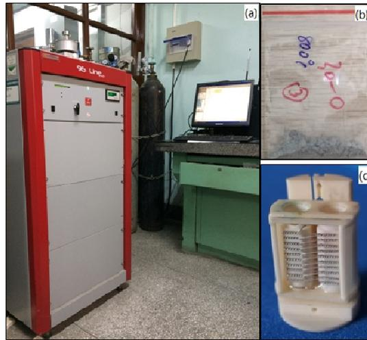
Fig. 2. Measurement of specific heat of coarse RCA concrete at elevated temperatures, (a) MHTC 96 Differential Scanning Calorimeter, (b) Concrete specimens, (c) Cell used for specific heat tests.
