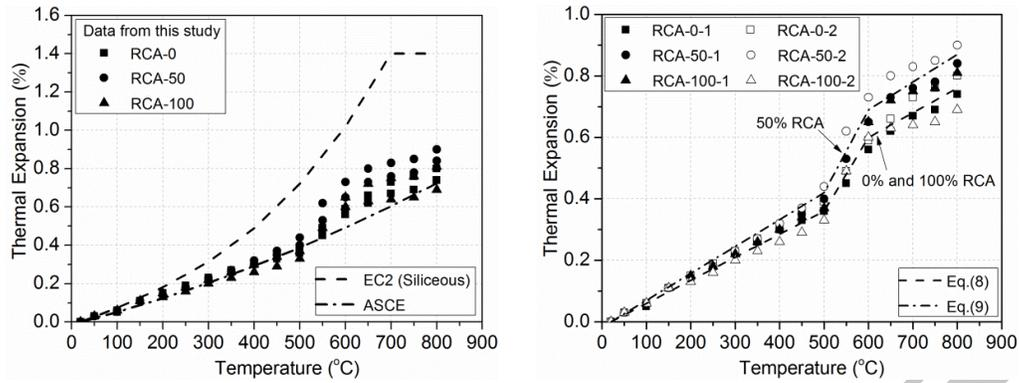
Fig.10. Comparisons of the thermal expansion of concrete specimens at elevated temperatures, (a) test results of this study, models of EC2 and ASCE, (b) test results of this study and corresponding regression expressions.
