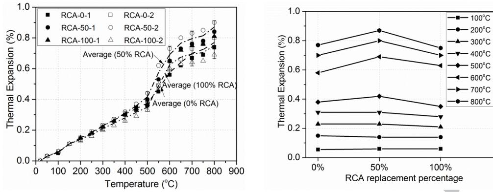
Fig. 9. Thermal expansion of coarse RCA concrete at elevated temperatures, (a) thermal expansion versus temperature, (b) thermal expansion versus coarse RCA replacement percentage.
