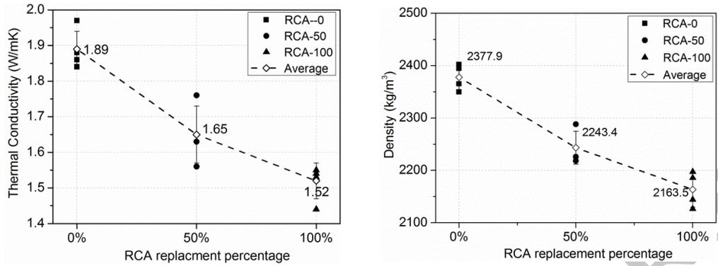
Fig. 4. Effect of coarse RCA replacement percentage on the thermal conductivity and density of coarse RCA concrete at room temperature.
