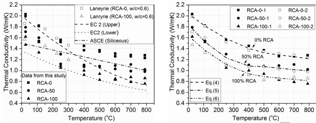
Fig.6. Comparisons of the thermal conductivity of concrete specimens at elevated temperatures, (a) test results of this study and Laneyrie, models of EC2 and ASCE, (b) test results of this study and corresponding regression expressions.
