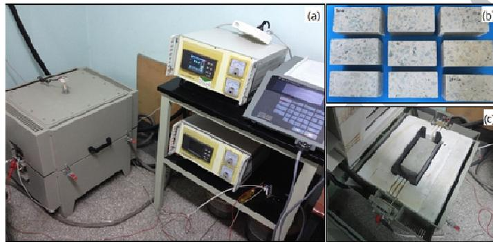
Fig. 1. Measurement of thermal conductivity of coarse RCA concrete at elevated temperatures, (a) Transient hot-wire device, (b) Concrete specimens, (c) Concrete specimen ready for thermal conductivity tests.
