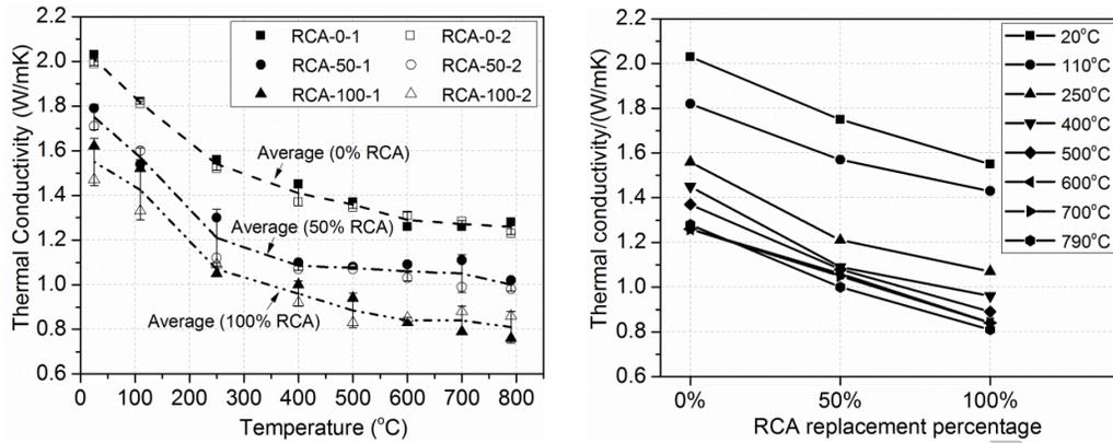
Fig. 5. Thermal conductivity of coarse RCA concrete at elevated temperatures, (a) thermal conductivity versus temperature, (b) thermal conductivity versus coarse RCA replacement percentage.
