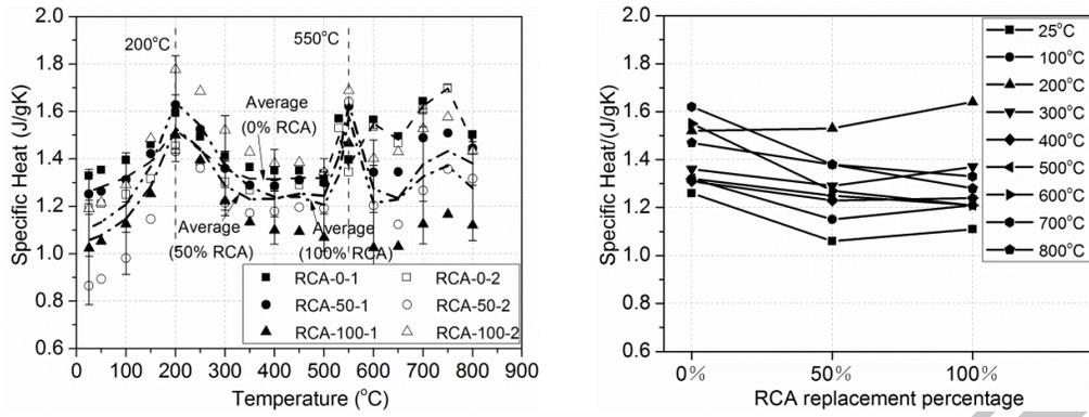
Fig. 7. Specific heat of coarse RCA concrete at elevated temperatures, (a) specific heat versus temperature, (b) specific heat versus coarse RCA replacement percentage.
