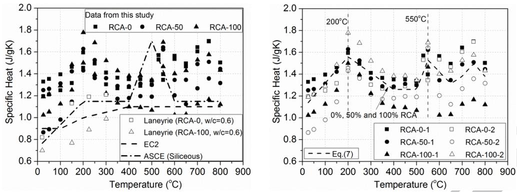
Fig.8. Comparisons of the specific heat of concrete specimens at elevated temperatures, (a) test results of this study and Laneyrie, models of EC2 and ASCE, (b) test results of this study and corresponding regression expressions.
