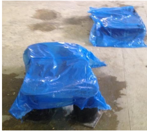
Figure 3 Cylinders Covered in Plastic Sheets for Curing
