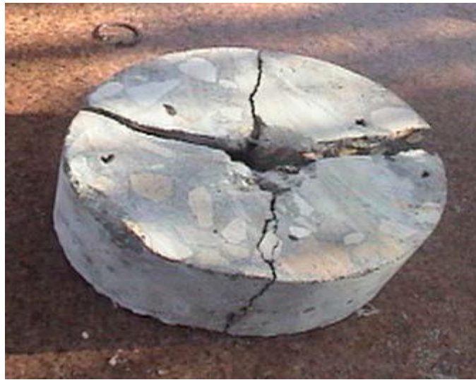
Figure 8 Plain Concrete Impact Failure
