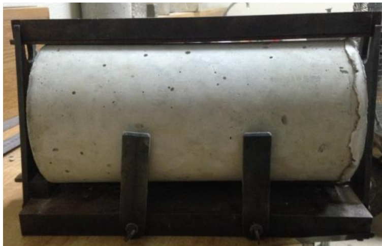
Figure 4 Cylinder Placed in the Steel Strips
