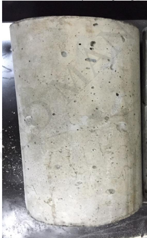
Figure 15: Rubberized Concrete Cylinders without Splitting After Failure
