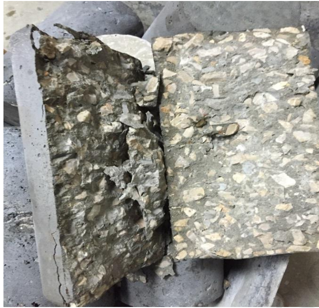
Figure 14 Non-Rubberized Concrete Cylinders Splitting into Two Halves.
