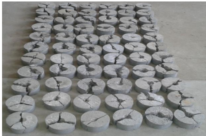
Figure 9: Portion of the Specimens Subsequently to Impact Load Failure
