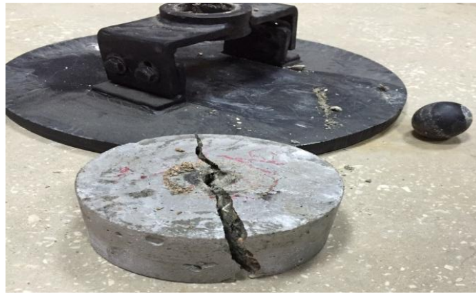
Figure 7 Rubberized Concrete Impact Failure
