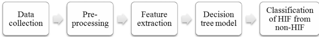
Fig. 1. The Proposed HIF detection method.
