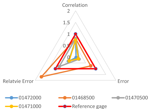
Fig. 8. The radar chart of correlation, relative error, and error of the BaSE-recommended gages and the original reference gage for site 8, normalized by corresponding metric of the reference gage.
