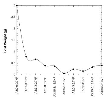
Fig. 3. Plot of lost weight in gravel-asphalt adhesion experiment for all samples.
