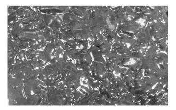
Fig. 2. Image of modified gravel covered with molten rubber-modified asphalt; the gravel surface was completely wetted by the asphalt.
