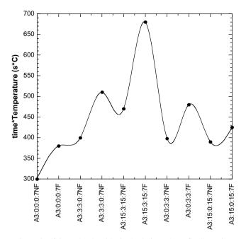
**Fig. 4.** Plot of the product  $(t \times T)$  in the ring-ball experiment for all samples.
