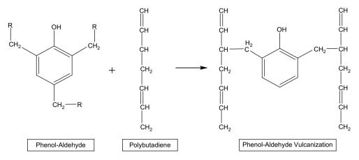
Fig. 1. Chemical reaction between PA resin and polybutadiene.
